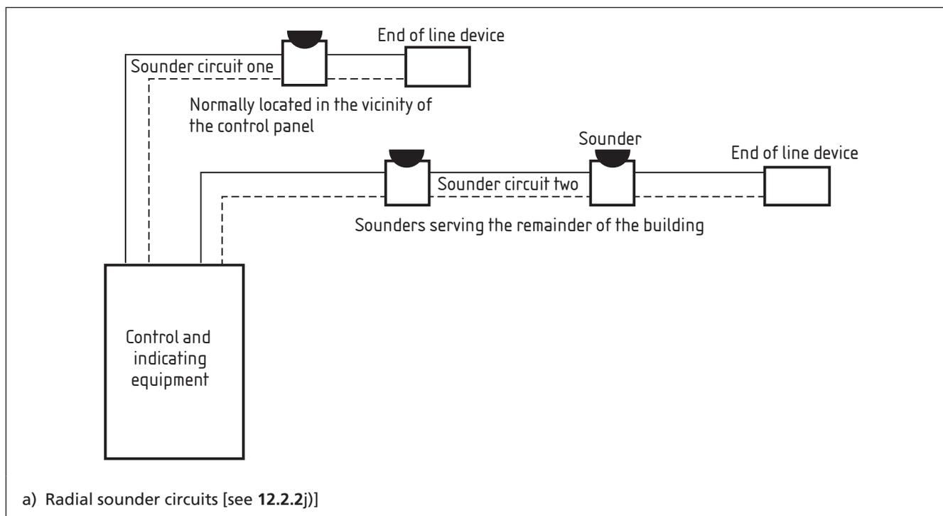
Figure 1 Sounder circuits (2 of 2)
