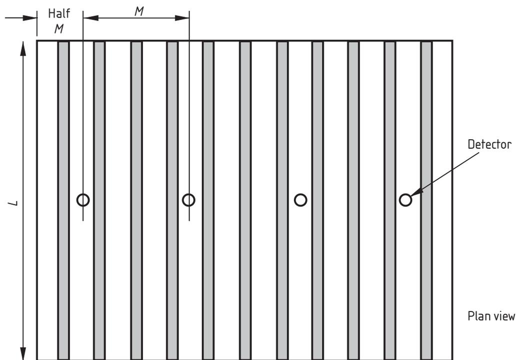
In this example beam downstands are greater than 10 % of ceiling height,  $H$ .  $H = 3$  m
