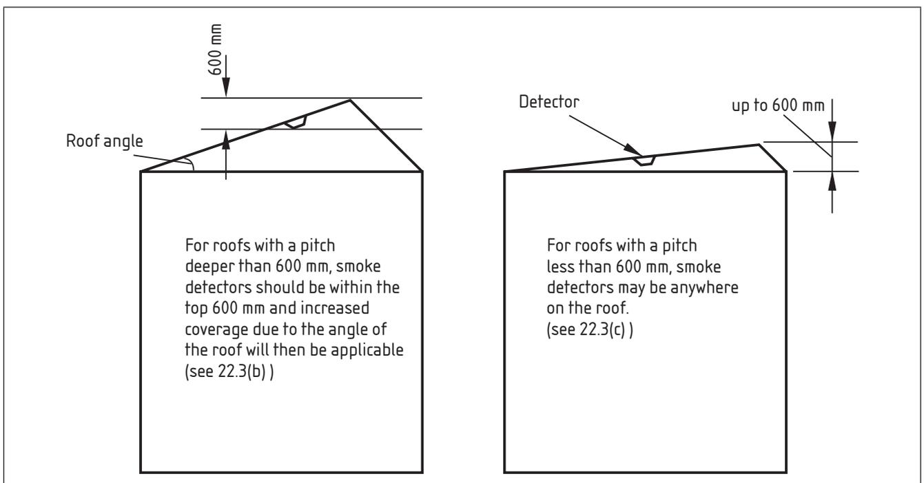
Figure 7 Detectors in top 10% of a void [see 22.3f)]
