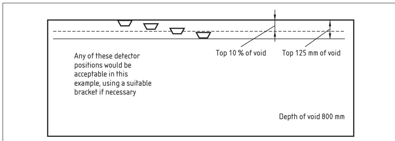
Figure 8 Proximity of detectors to ceiling fittings [see 22.3h)]
