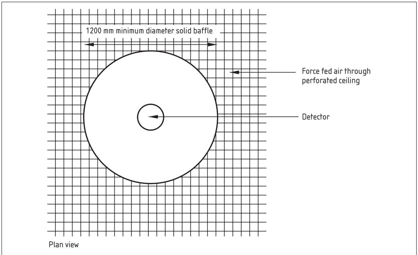
Figure 12 Clear space around a detector [see 22.3o]
